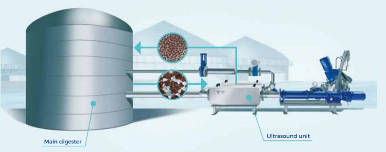
Taking into account specific substrate properties, the ultrasonic disintegration system can be integrated into the existing process technology in a variable and uncomplicated way and without affecting operating processes.
