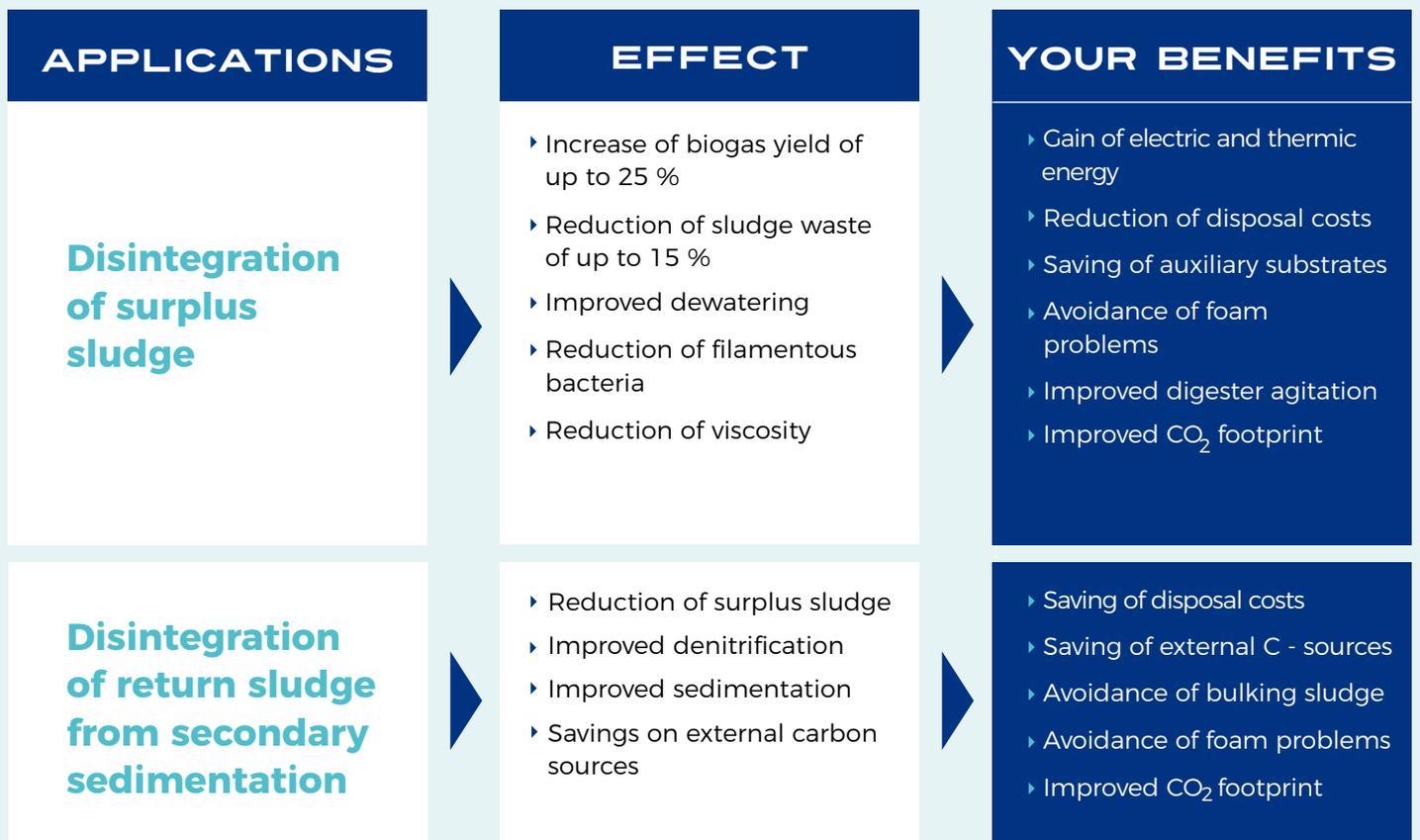
The problem of the fiber bacteria *Microthrix parvicella*, the typical root cause of foam and bulking sludge, is significantly reduced through ultrasonic treatment.
