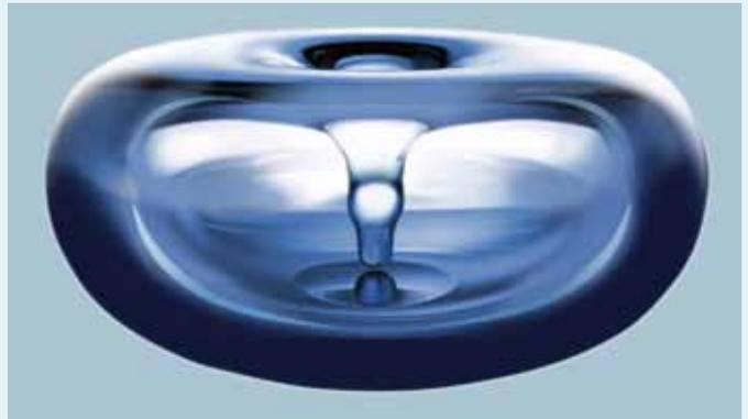
**Multiply enlarged cavitation bubble immediately before implosion.**
